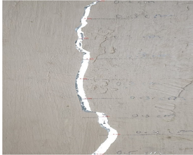
Figure 6 Crack width validation: manual measurements (cm) versus automated results (mm)
