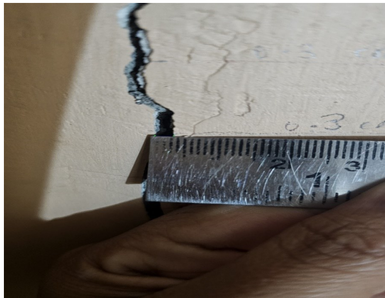
Figure 7 Manual measurement of crack width using a physical ruler (scale in centimeters) for calibration and validation of the pixel-to-millimeter conversion factor.
